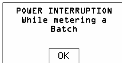
Figure 44: Typical “Power Interruption” Alarm Screen
